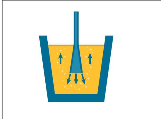
Fig 3 Magnesium mono-injection process, with evaporation chamber
