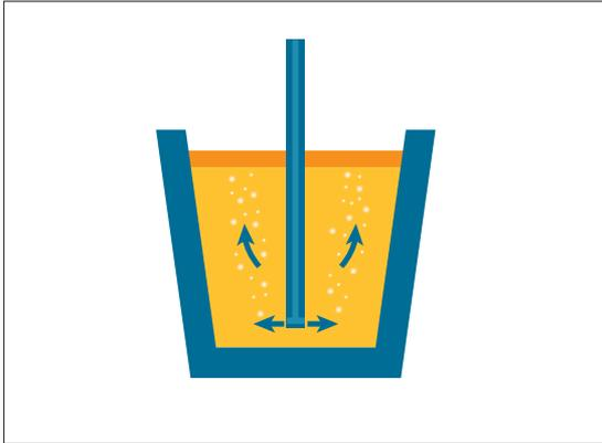
Fig 4 Co-injection process, with T-shaped lance exit
