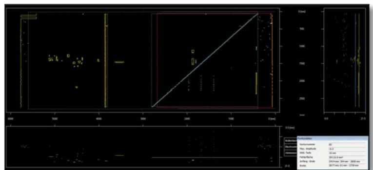
Ⓐ Fig 5 Sample view of AES user interface showing results from a test plate with oblique and transverse notches
