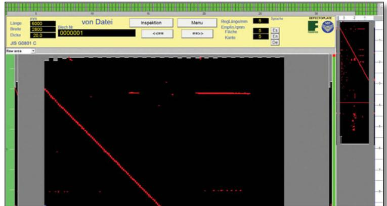
Ⓐ Fig 4 Sample view of DEU user interface showing results from a test plate with oblique and transverse notches
