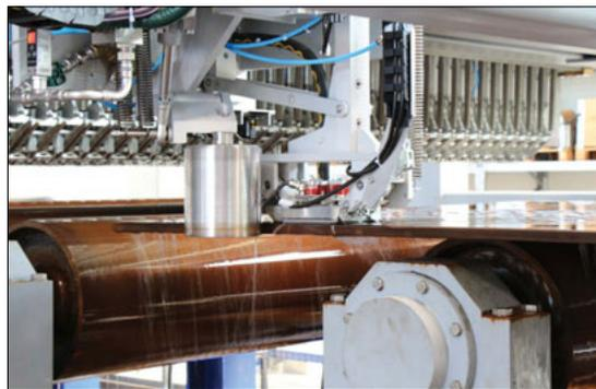
Ⓐ **Fig 2 Ultrasonic testing system in operation, showing carriage D for simultaneous longitudinal edge inspection**
