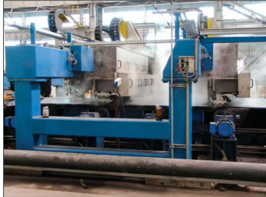
Ⓐ **Fig 1 Ultrasonic testing system in operation, showing body inspection carriages A and B for full coverage of plate body in one run**
