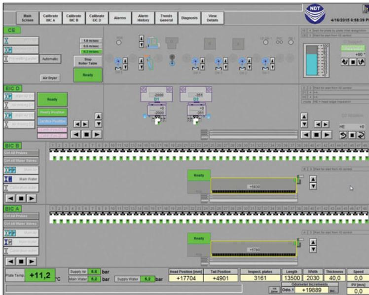
Fig 3 Sample view of WinCC user interface for a testing system designed for inspection from above
